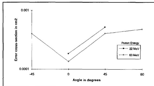
Figure 6 REC error cross-section vs. beam incidence angle
