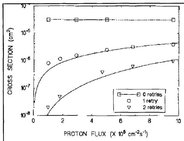
Figure 8 1773 REC error cross-section vs. flux for 0,1,2 retries
