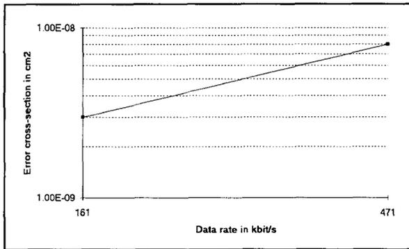
Figure 7 1773 TX error cross-section vs. data rate (63 MeV)
