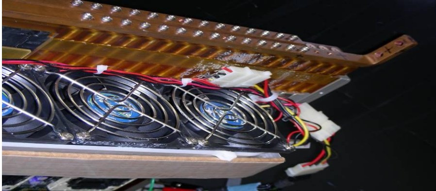
Figure 3. Power Supply Bus Bars above the Cooling Fans
