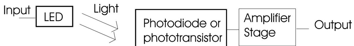
Figure 1 Typical Optocoupler Block Diagram
