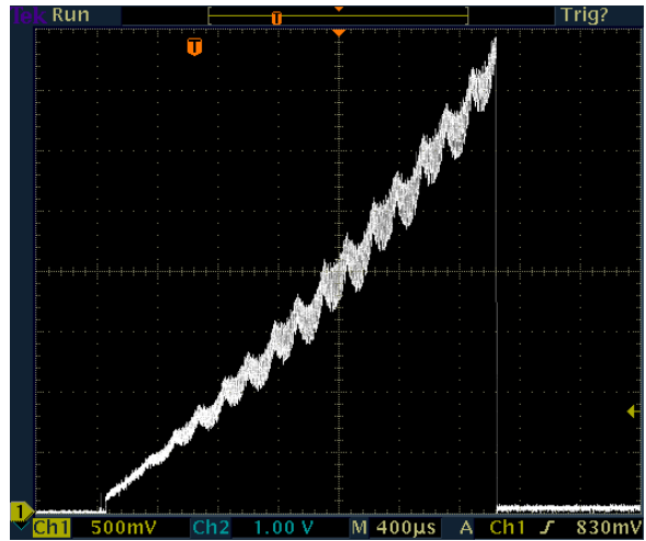
Figure 15-LTC1657 transfer curve after 10k rad(Si)
