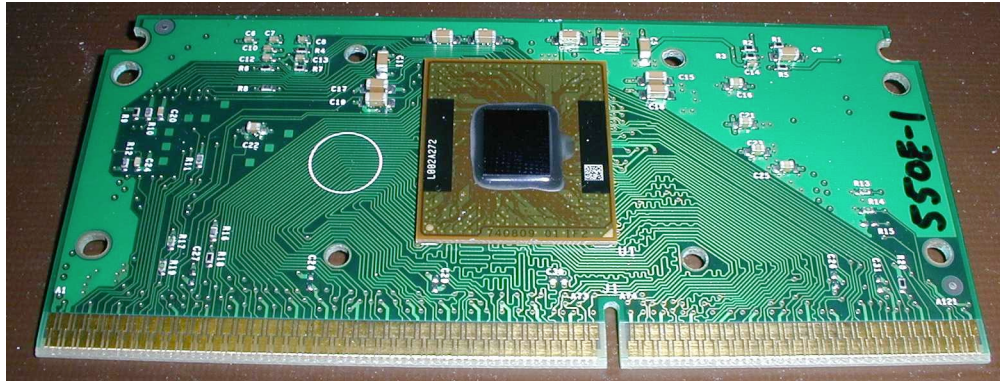
Figure 8. The DUT PCB, showing the OLGA, and the epoxy fillet around the die.
