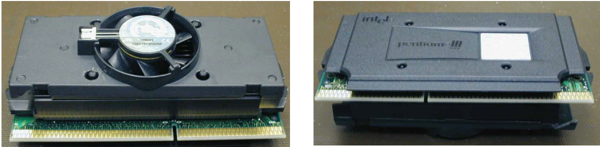
Figure 6. Photographs of Pentium III SC242 processor showing fan side and front side.
