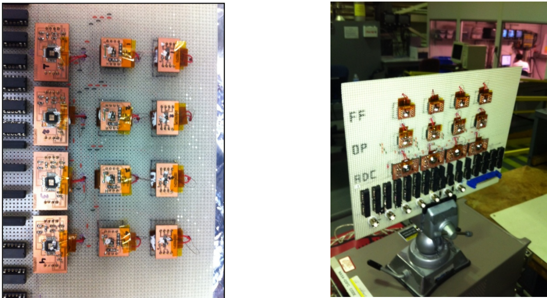
Figure 3: Test board configuration for the SEL test of the NC7SZ74 D flip-flop. The NC7SZ74 is located on the right row in the left image and the top row in the right image. The other parts on the test board were evaluated during the same run, but are not covered in this report.
