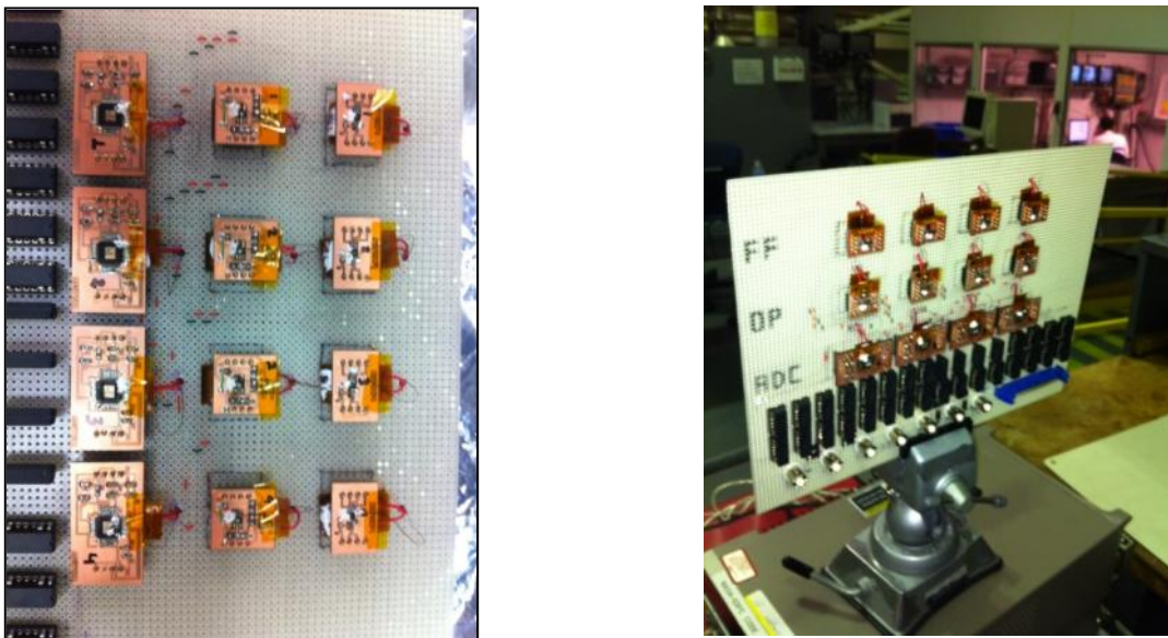
Figure 3: Test board configuration for the SEL test of the LTC2054HV operational amplifier. The LTC2054HV is located on the middle row in the left image and the middle row in the right image. The other parts on the test board were evaluated during the same run, but are not covered in this report.
