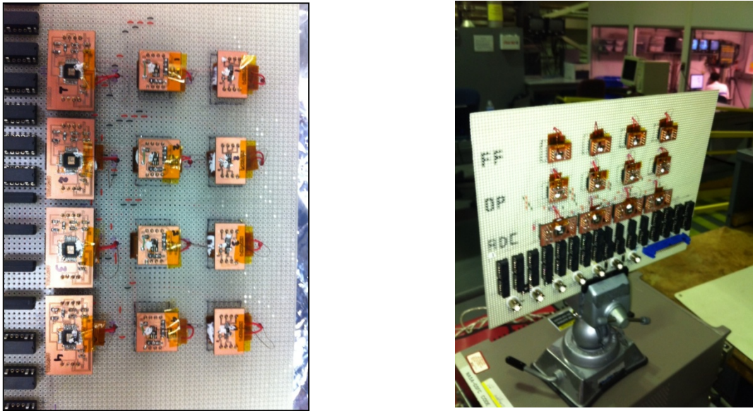
Figure 3: Test board configuration for the SEL test of the ADS7881 SAR ADC. The ADS7881 is located on the left row in the left image and the bottom row in the right image. The other parts on the test board were evaluated during the same run, but are not covered in this report.
