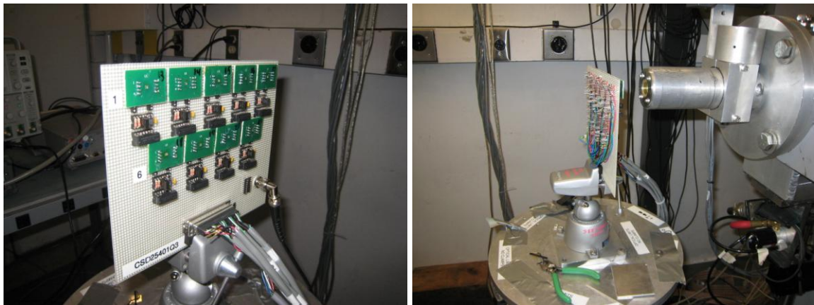
Figure 4. Left: Frontside of board with 9 individually-selectable DUTs mounted. Right: Backside of test board positioned in the beam line.
