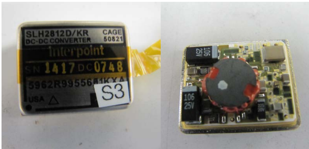
Figure 3. SLH2812D cover and internal circuitry test at LBNL
