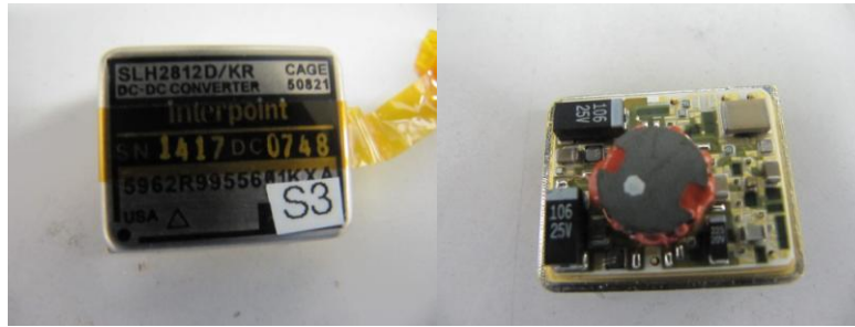
Figure 3. SLH2812D cover and internal circuitry test at LBNL
